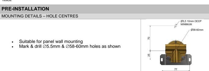
Tools required: Power drill, spanner or adjustable cresent and hex key.
